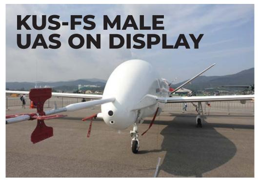
A prototype of the high performance | KUS-FS Medium Altitude Long Endurance (MALE) Unmanned Aerial System (UAS) being developed by Korean Air and LIGNex1 is being showcased at the outdoor static display. The 3m tall KUS-FS made its first flight in 2012. This is the first show appearance for the MALE UAS type, which is 13m in length and has a 25m wingspan.
