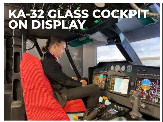
Russian Helicopters is displaying an avionics demonstrator of the proposed 'glass cockpit' upgrade available for the Ka-32 helicopter. This modernisation effort will involve the replacement of analogue gauges in the cockpit with three LCD displays, ranging from 14-17", based on customer requirements. Also included are terrain avoidance systems, a flight computer and a digital autopilot.
