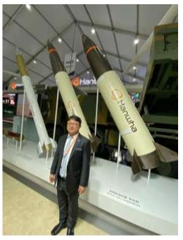
Chunmoo 2 (400 mm) and two rounds of the new Chunmoo 3 or KTSSM with 600 mm (24 inch diameter). The company says the new weapon has a more powerful warhead, longer range and greater resistance to jamming than the other versions of Chunmoo. According to Hanwha, their guided rocket is used as a "bunker buster" solution by the army because of its penetrator warhead.
