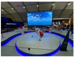
speed of 250 km/h and at a maximum altitude of 14,763 ft. It measures 3 m in length and approximately 5 m wide. It has a maximum take-off weight of 210 kg. It can carry a 30 kg payload, such as a stabilized forward looking infra-red (FLIR) and have a 200 km radius of action with an endurance of 5-6 hours.
